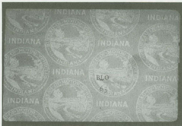
The letters "BLO" and the number "63" have been applied to the top of a security-laminated license. These alterations show up immediately under retroreflective light.
