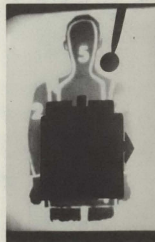
Figure 13—Bullet strike will be high and right when the front sight is misaligned high and right with respect to the rear sight.
