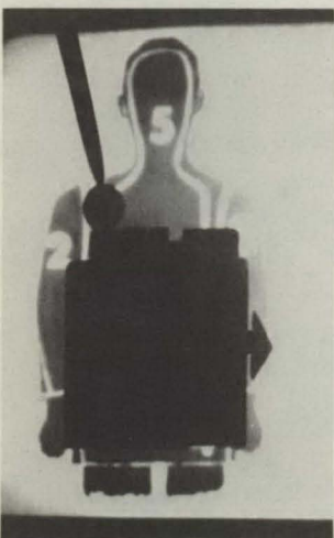
Figure 10—Bullet strike when the front sight is aligned level with the rear sight but off center to the left.
