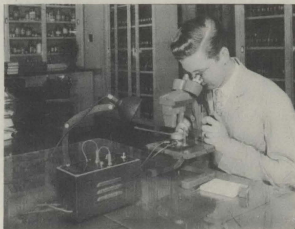
Figure 2.—Micro melting point apparatus assists in identifying unknown substances isolated from organs of poisoned victims.
