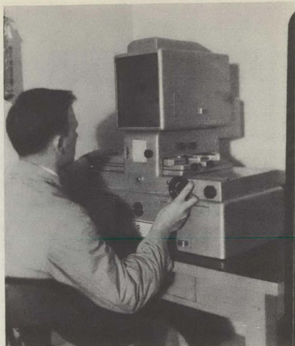
Figure 4.—The densitometer interprets the photographic plate obtained in a spectrographic analysis.
