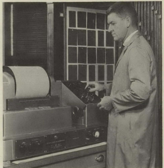
Organic vehicles in paint may be identified and compared by use of the infrared spectrophotometer.
