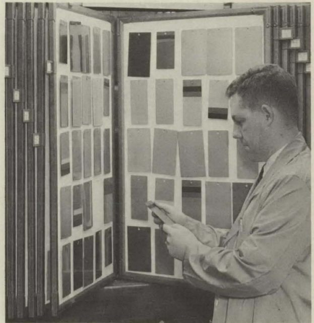
By reference to panels in the National Automotive Paint File, the Laboratory examiner can often associate a paint chip with a particular make car.
