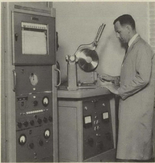
Pigments and extenders in paint may be identified by a study of X-ray diffraction patterns produced by the X-ray diffractometer.
