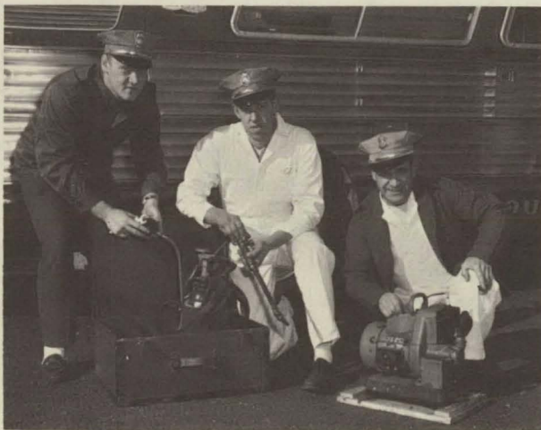
Emergency equipment utilized by the North Penn Goodwill Service includes oxygen tank, acetylene torch and emergency generator, wrecking crowbar, wire cutters, and ax.
