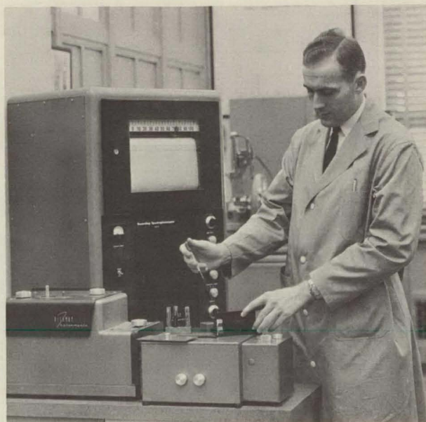
The spectrophotometer measures color and makes a graph. It is used to identify and compare dyes.
