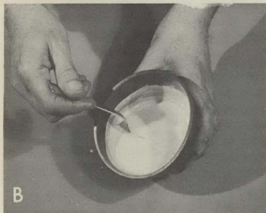
Figure 7. Proper mixing of plaster of paris: (a) powder added to water; (b) allowed to soak for 15 to 30 seconds; (c) should be free of bubbles and flow evenly.
