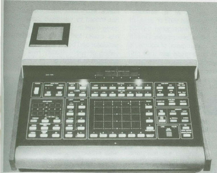
This microprocessor enables the operator of the S.M.E. simulator to control completely the settings to which an officer is exposed.
